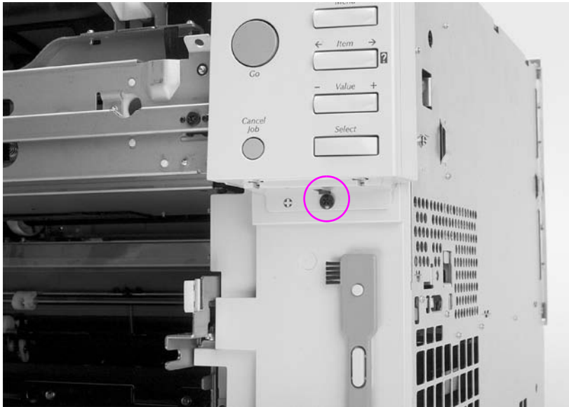
Figure 6-11 Control panel removal and replacement
