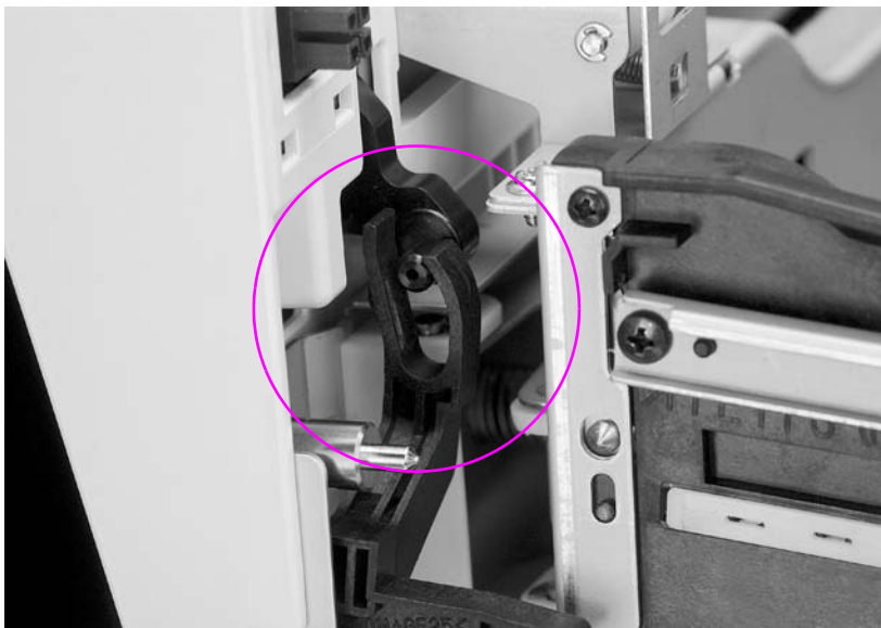
Figure 6-8 Drum drawer (top drawer) cover tabs and levers
